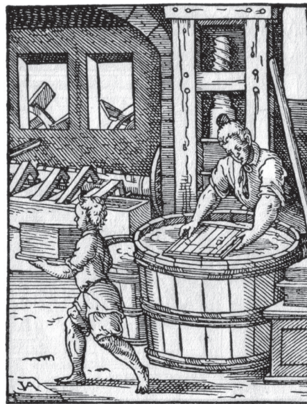
Figure P1.5 Paper making—Suspending linen fibers in water, and then pressing the fibers in a layer against a screen, is the technique for making paper, a much cheaper medium for books than parchment. Woodcut by Jost Amman, 1568.
